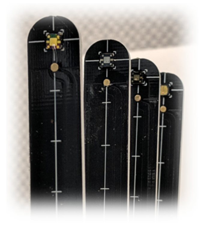
Fig. 3. Detector mount. The detector frames made out of printed circuit boards with the detector centered at the tip of the frame.
